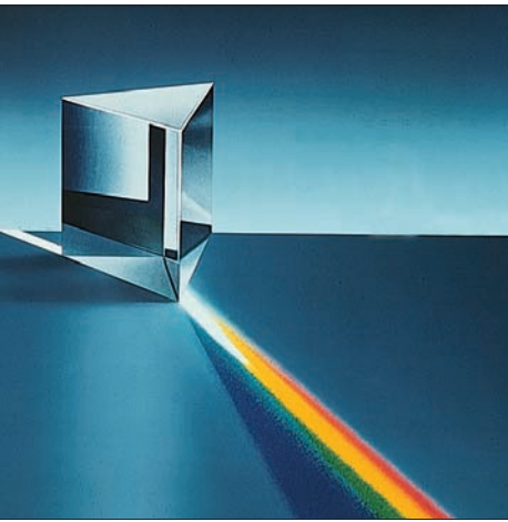
FIGURE 2-1 When white light passes through a prism, a full optical spectrum results, with different colors bent by different amounts.
